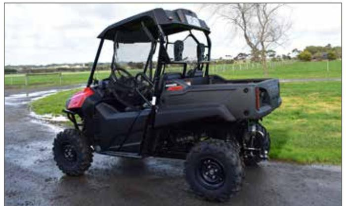
An example of a side-by-side utility vehicle with fitted seat belts and rollover protection.
